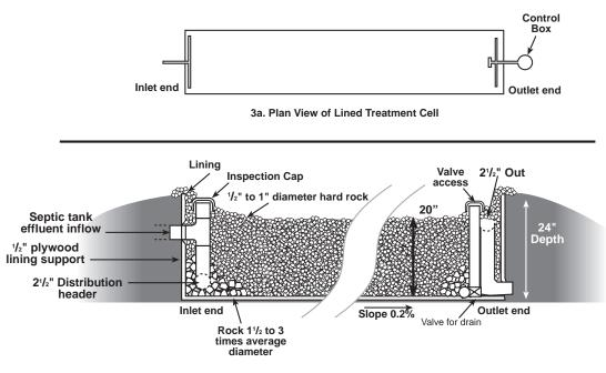
3b. Longitudinal Section of Lined Treatment Cell
