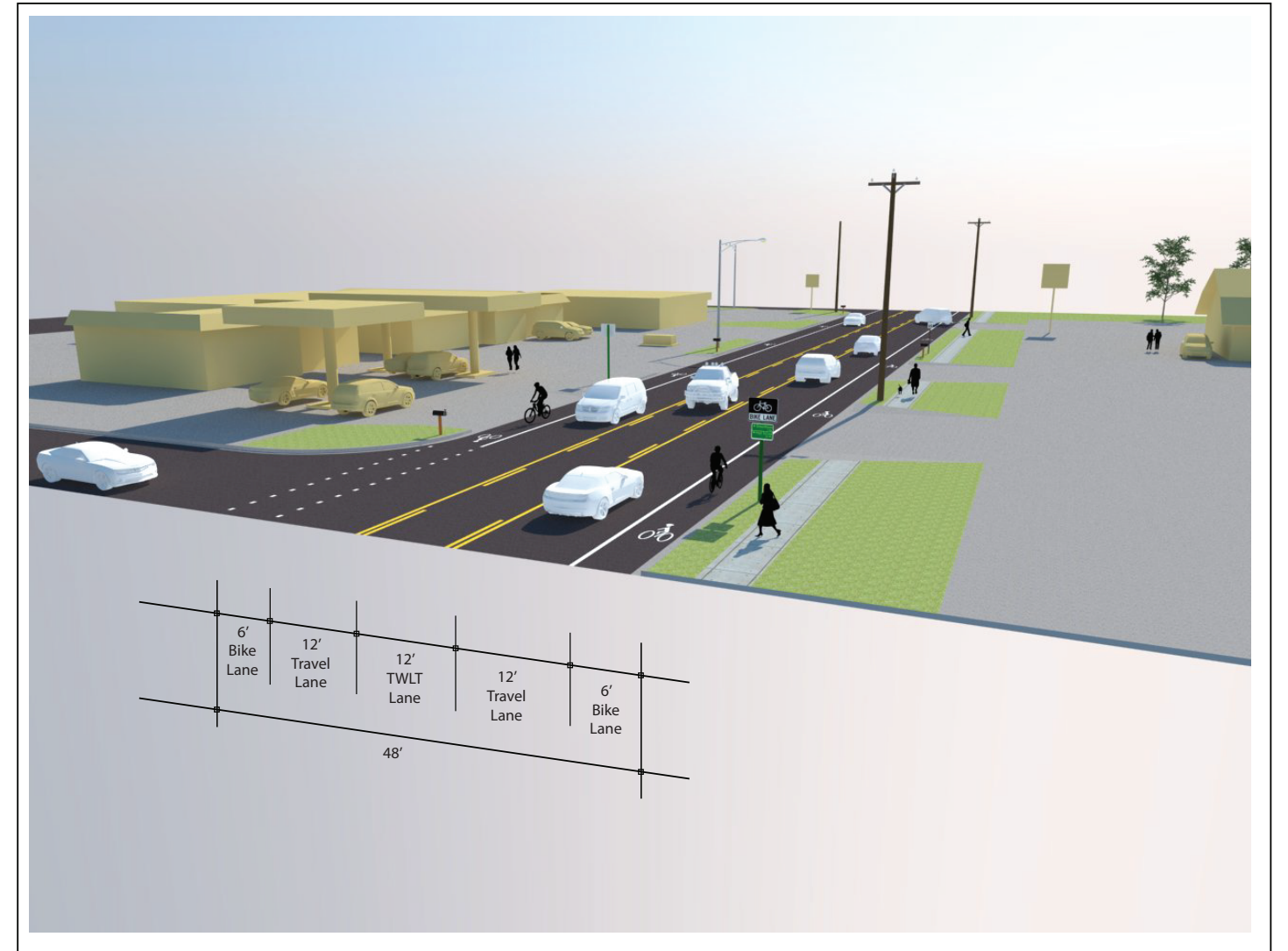
Figure 6.5 - N Meridian Road., near W 5th St. - Rightsizing from Four-Lane Section to Three-Lane Section with Bicycle Lanes (No On-Street Parking)
